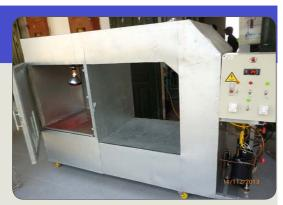
exposed to the heated air with relative humidity of drying air RH = 20 - 40 %. The study shows that dried shallot leaves have high quality and high efficiency.
